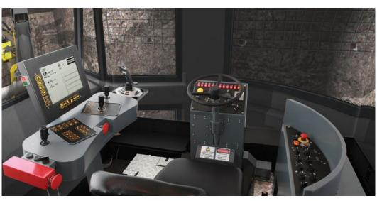
> Physically accurate vehicle cab The trainee operator executes all tramming, drilling and bolting tasks from a highly accurate replica of the cab interior. The seat is surrounded by fully functional controls including steering wheel, switches, gauges, levers, pedals and joysticks.
